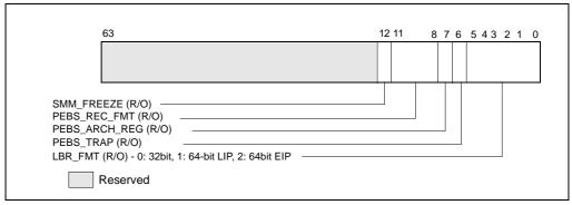
Figure 30-29. Layout of IA32\_PERF\_CAPABILITIES MSR
