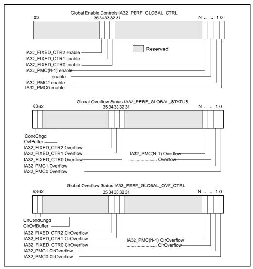
Figure 30-8. Layout of Global Performance Monitoring Control MSR
