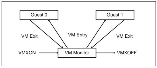
Figure 20-1. Interaction of a Virtual-Machine Monitor and Guests
