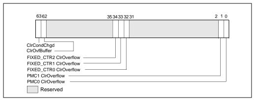
Figure 30-12. Layout of MSR\_PERF\_GLOBAL\_OVF\_CTRL MSR
