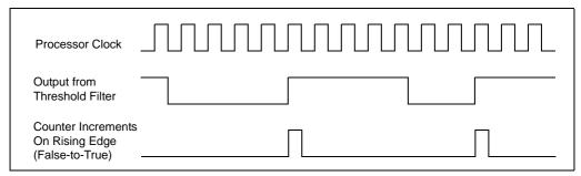
Figure 30-26. Effects of Edge Filtering
