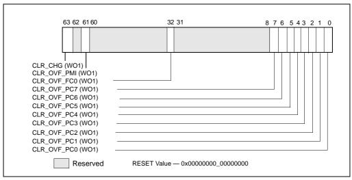
Figure 30-19. Layout of MSR\_UNCORE\_PERF\_GLOBAL\_OVF\_CTRL MSR
