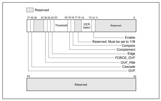
Figure 30-25. Counter Configuration Control Register (CCCR)
