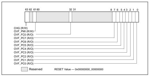
Figure 30-18. Layout of MSR\_UNCORE\_PERF\_GLOBAL\_STATUS MSR
