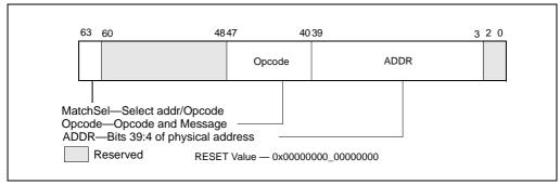
Figure 30-22. Layout of MSR\_UNCORE\_ADDR\_OPCODE\_MATCH MSR
