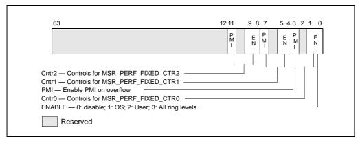
Figure 30-9. Layout of MSR\_PERF\_FIXED\_CTR\_CTRL MSR
