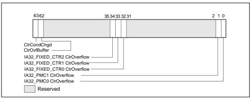
Figure 30-5. Layout of IA32\_PERF\_GLOBAL\_OVF\_CTRL MSR
