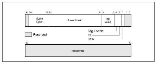
Figure 30-23. Event Selection Control Register (ESCR) for Pentium 4 and Intel Xeon Processors without Intel HT Technology Support
