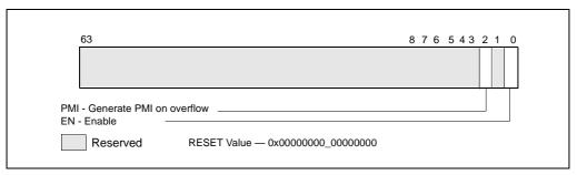
Figure 30-21. Layout of MSR UNCORE FIXED CTR CTRL MSR
