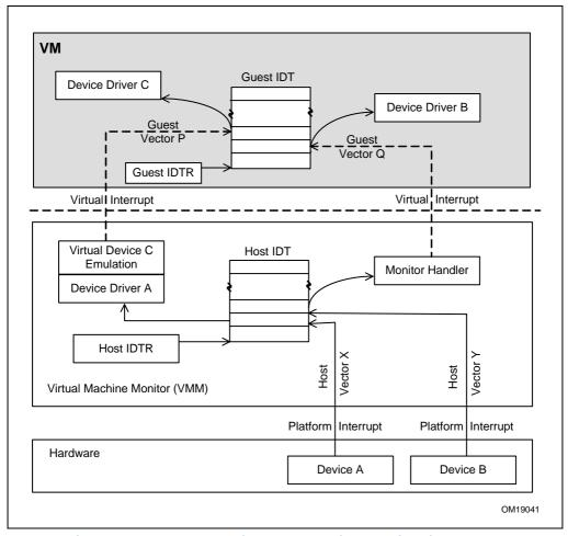
Figure 29-1. Host External Interrupts and Guest Virtual Interrupts
