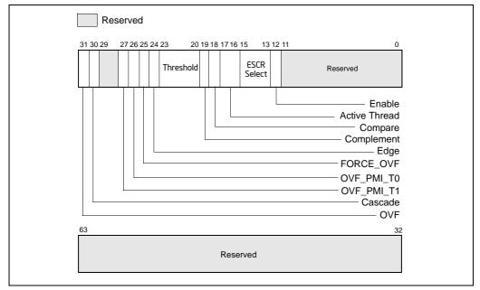
Figure 30-28. Counter Configuration Control Register (CCCR)
