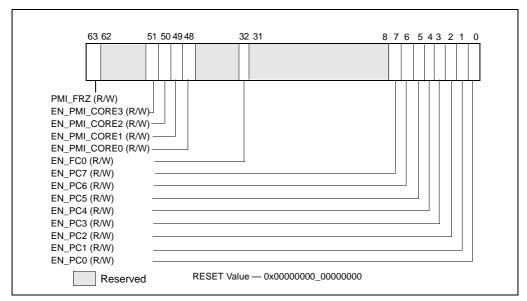
Figure 30-17. Layout of MSR\_UNCORE\_PERF\_GLOBAL\_CTRL MSR
