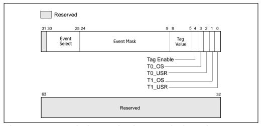
Figure 30-27. Event Selection Control Register (ESCR) for the Pentium 4 Processor, Intel Xeon Processor and Intel Xeon Processor MP Supporting Hyper-Threading Technology
