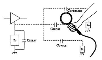
$$\label{eq:constraint} \begin{split} & \text{When } Z_G \text{ is large and } C_{\text{STRAY}} \text{ is small}, \\ & \text{C}_{\text{OPERATOR}}, \, C_{\text{PROBE}}, \, C_{\text{CABLE}} \, \text{can be significant} \end{split}$$
