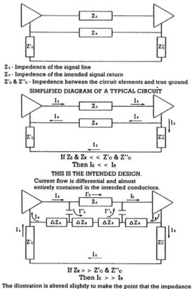
The illustration is altered slightly to make the point that the impedance of the return line is distributed and that there is a distributed capacitance between the signal lines. If  $Z_n >> Z'_c \& Z''_c$ then the signal will be carried on both the signal and return lines. The return current will be shunted outside the circuit.
