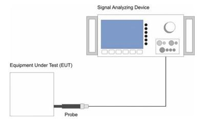
**2.** Connect a coaxial cable from the probe to the signal analyzing device; typically, an oscilloscope or spectrum analyzer.
