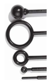
The probes provide a fast and easy means of detecting and identifying signal sources that could prevent a product from meeting federal regulatory requirements. This set is a convenient and inexpensive tool for extending the capability of a spectrum analyzer, oscilloscope, or signal generator.
