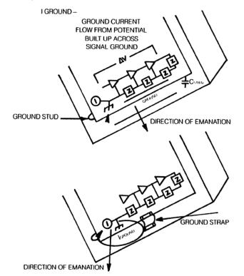
The placement of ground straps changes the geometry of the radiating current loop. A ground strap may reduce the signal, but it will also redirect it. To properly assess the modification, the perimeter of the unit must be scanned. The more distant measurement points may lose the signal into the system noise; a given solution may only redirect the beam. Especially with narrow beam problems, solutions frequently only shift the beam so that it radiates in a different direction.
