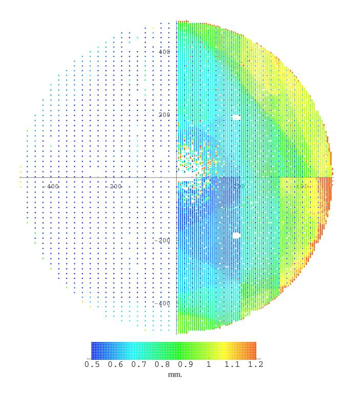
Top of plot is North. The targets around the central hole have been contaminated by fungus or dirt. The tiling of the pictures can be seen. Note that the tieback targets have lower uncertainty.
