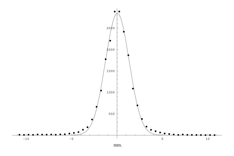
Histogram of 19489 points, 132 points off scale. Width of fitted gaussian: 1.8 mm. Included tieback points cover the entire reflector.
