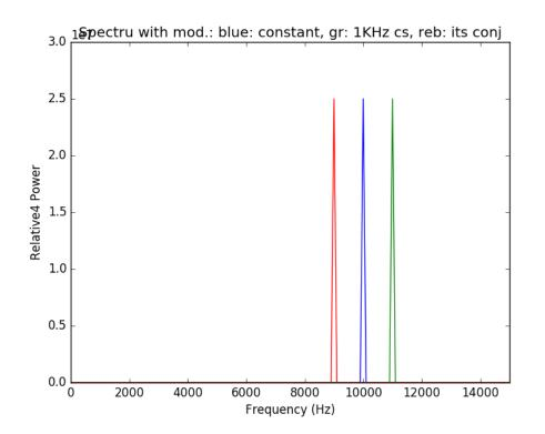
If we want to generate two frequencies in such a way that the spectrum is not symmetric (for example the Carlson/Djuth two frequency experiment), it would be easier to generate them at rf and then bring them to baseband with the baseband mixer. We could generate two complex sinusoids at baseband, but it seems easier to generate two real sinusoids at rf.
