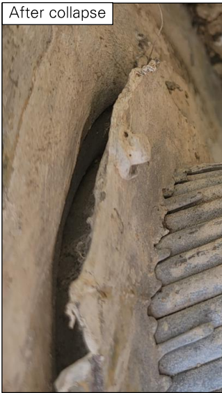
Figure 31: Cable slip at socket M12W_P.
