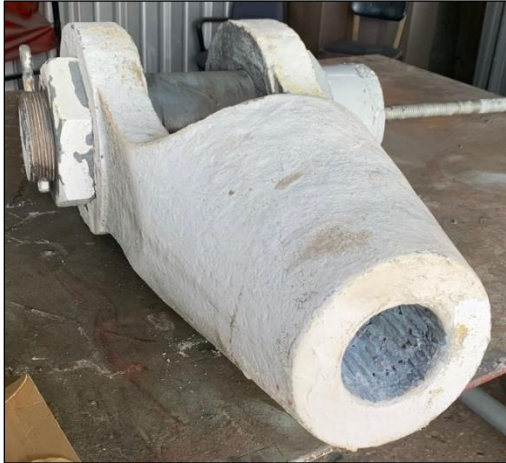
Figure 2: Socket M4N_T recovered from Tower 4 after M4N failure (photo: WJE).
