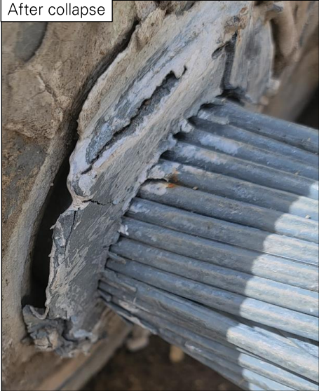
Figure 30: Cable slip at socket M12E_P.
