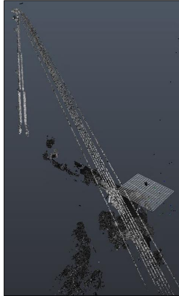
Figure 2: Tower 12 backstays in August 2020 laser scan.
