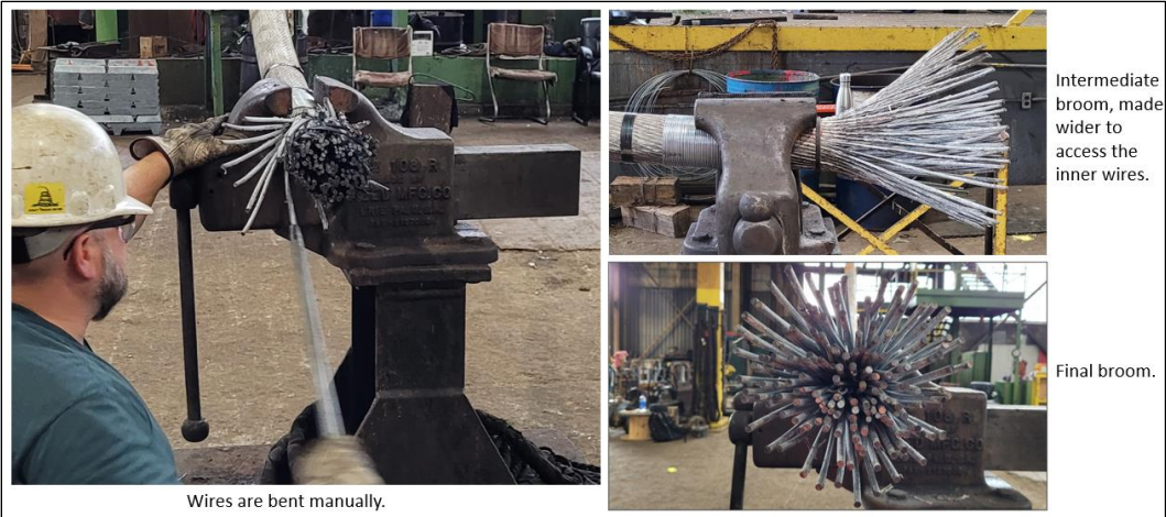
Figure 3: Manual wire brooming.
