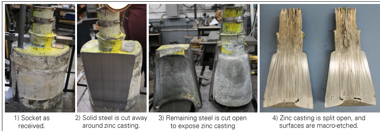
Figure 10: Initial processing of socket B12W_G (photos: Socotec).
