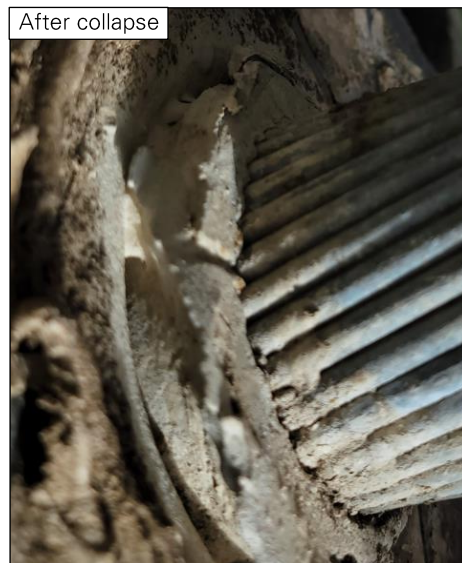
Figure 28: Cable slip at socket M8N_P.
