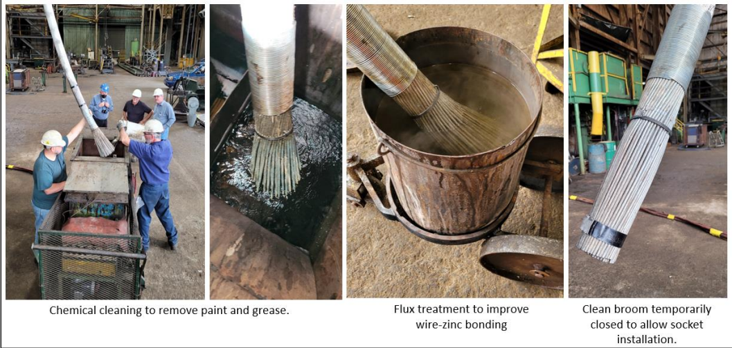
Figure 4: Wire broom cleaning.
