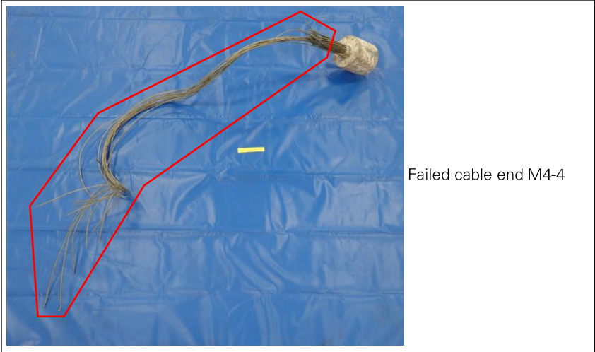
Figure 2: Socket M4-4_T with multiple M4-4 wires fractured outside of socket (photo: Socotec).
