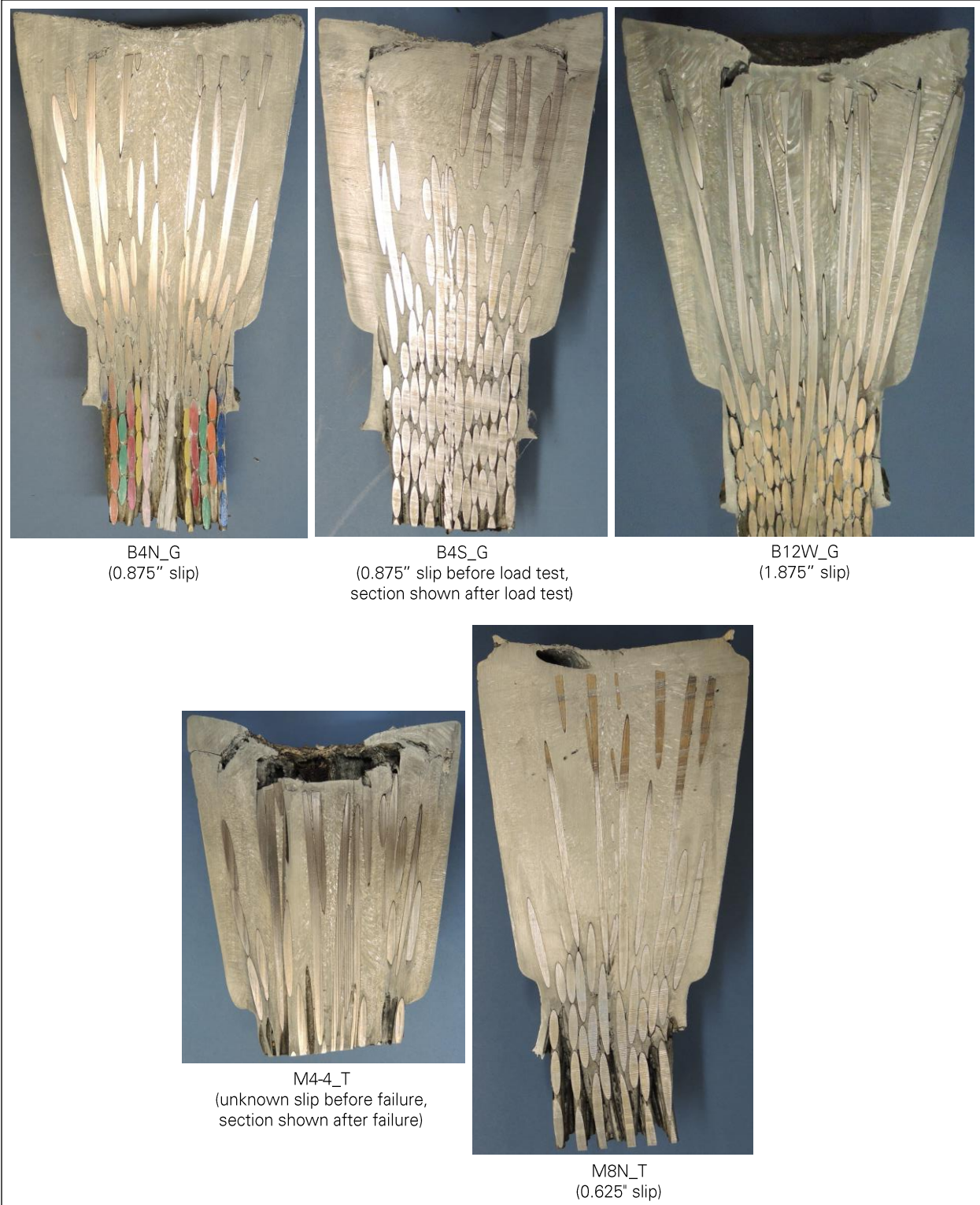
Figure 11: Macro-etched transverse sections of socket zinc castings (photos: Socotec).
