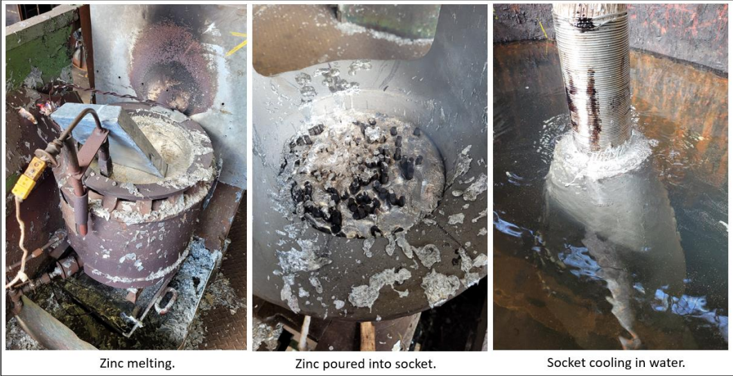
Figure 6: Zinc casting and socket cooling.
