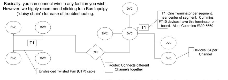
Note: Although LonMaker says that you can have 2 segments to a channel, we are not confident in this, so stick to a maximum of 64 devices, 1 segment per channel
