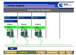
The main menu screen displays the equipment monitored by the iWatch location that is connected. It also displays the basic status of each component, such as whether it is operating or what sources are available. The user may click on a component that is displayed or one of the tabs at the bottom of the screen to navigate to other system displays. When a warning or shutdown condition is present on any equipment monitored, a warning (yellow) or shutdown (red) banner is displayed on the screen.
