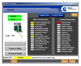
This display emulates operation of a genset annunciators, providing status condition on one screen for the major components in the system. The screen also allows manual starting and stopping of the generator set for operators that are authorized to perform that function.
