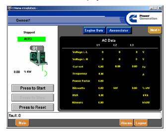
The generator set AC data display screen provides information on the current AC voltage, current, frequency, power factor, kW, kVA, and kVAR output of the generator set monitored. The screen also allows manual starting and stopping of the generator set for operators that are authorized to perform that function. For paralleling applications other screens may be provided that show generator set state, breaker positions, and other information.
