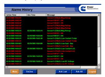
The fault information display provides the user with a date and time-stamped remote indication of alarm conditions that have occurred at a site. The data displayed is the name of the device on the network and the name of the alarm condition that occurred. Conditions that have been acknowledged are shown in green text, and those that have not are shown in red.
