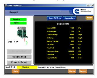
The generator set engine data display provides detailed information on the state of the engine, including speed, oil pressure, coolant temperature, oil temperature, battery voltage, fuel rate and total fuel consumed (when available), engine running hours, kW hours, and number of starts. Units of measurement are configurable for either US Standard or Metric values. The screen also allows manual starting and stopping of the generator set for operators that are authorized to perform that function.
