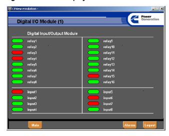
Digital I/O modules on the PowerCommand LonWorks network allow the network to monitor discrete inputs from fuel systems and other equipment, so that a user may see their status (green-normal, yellow-warning, or red-shutdown) and control them from a remote location.
