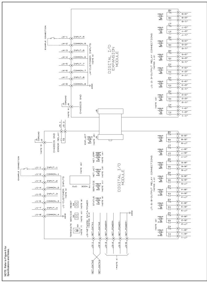
FIGURE 5. DIGITAL I/O MODULE INTERCONNECT WIRING DIAGRAM
