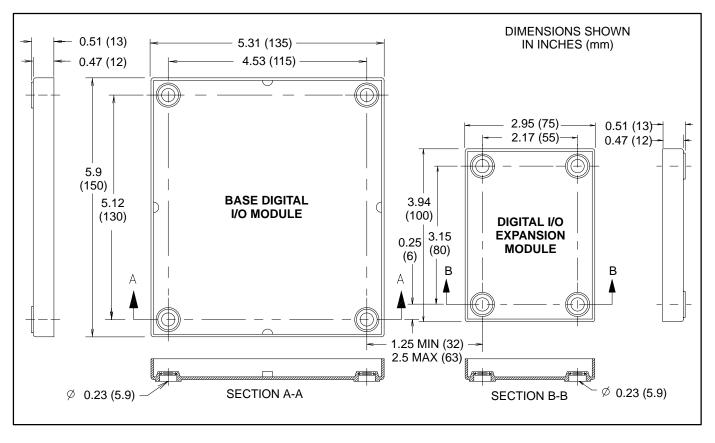
FIGURE 3. DIGITAL I/O MODULE FOOTPRINTS
