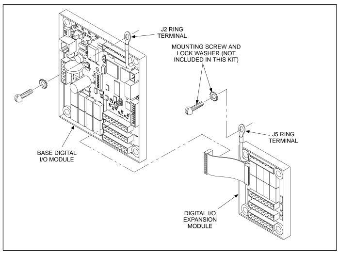
FIGURE 4. DIGITAL I/O MODULE INSTALLATION
