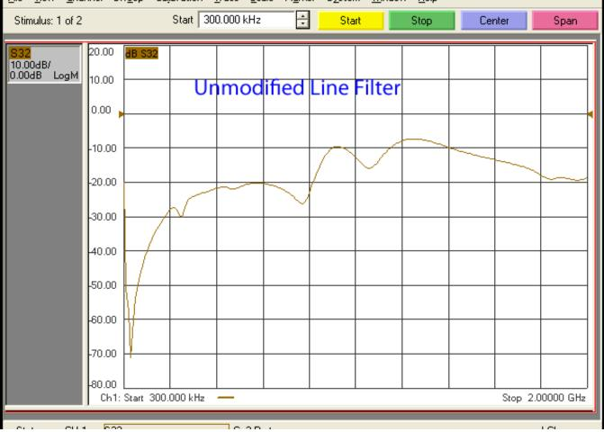
In an attempt to improve the performance in the low/mid L-band regime, a 1000pF capacitor with minimal lead lengths was added as shown on page 5. The VNA test results are shown on page 6.
