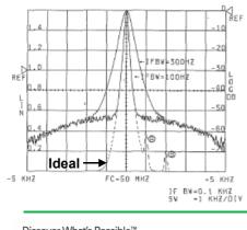
For the local signal source, the dotted line spectrum is the ideal. However, it actually has sideband noise like the solid line. Masking occurs by the sideband noise when there is a nearby A or B signal and it is not possible to detect it.
