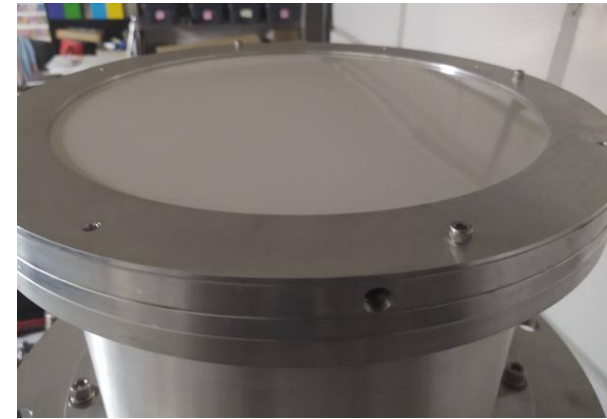
FLAT Radome Installed
