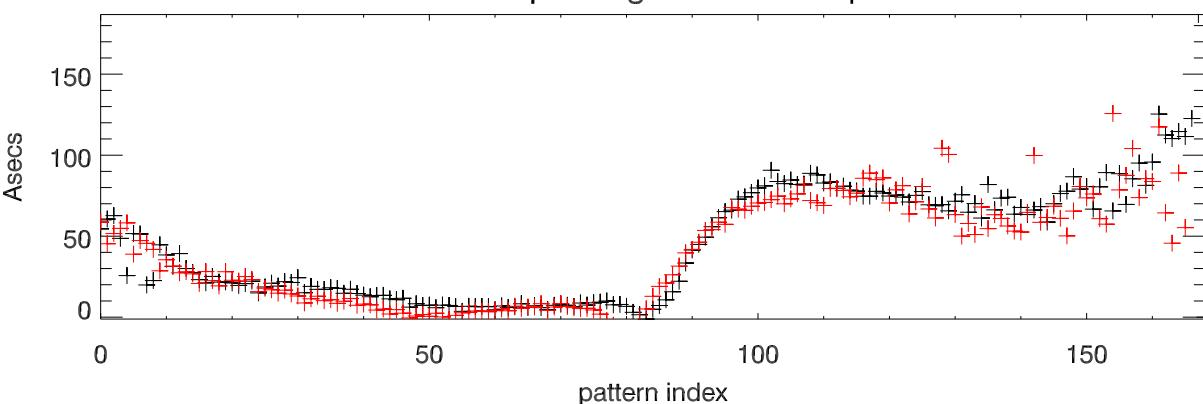
Crab EI pointing errors vs elevation
