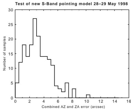
Fig. 7: Distribution of measured pointing residuals, following installation of the new pointing model. The standard deviation is 3.7 arcseconds, with a 95<sup>th</sup> percentile value of 7.7 arcseconds.
