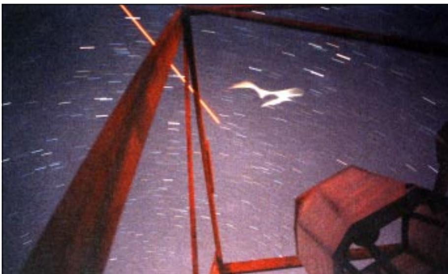
The Arecibo Observatory sodium resonance lidar's laser and telescope frame the luminous cloud from a TMA release during the Coquí II sounding rocket campaign in February-March. See the article on page 4.
