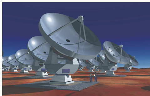
The ALMA array is designed to operate as 64 "independent" single dish telescopes, as well as a 2016-baseline interferometer
