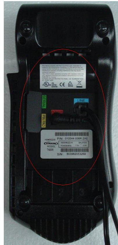
Figure 2: T4205 rear - hot spot.
