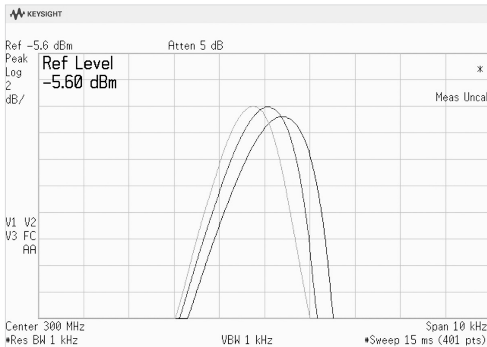
Figure 2-14. Sweeping an analyzer too fast causes a drop in displayed amplitude and a shift in indicated frequency
