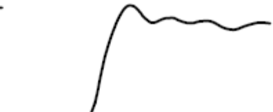
Signal with a long ground lead
