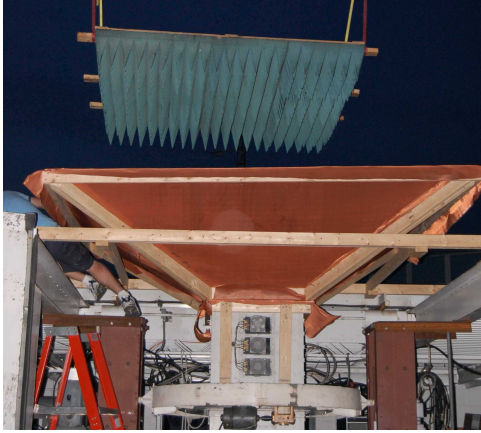
Fig. 2.— Ground shield and PAF in sky noise measurement facility with absorber being lowered over the array for T_{\text{hot}} measurement measurement (July, 2008).
