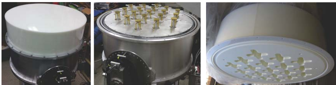
Figure 5: Left: Successfully tested shield-modified AO-19 cryo-PAF with the HDPE top hat over the three layers of Rohacell foam. Center: Shield-modified AO-19 cryo-PAF after removing the three layers of foam above the dipoles and the HDPE top-hat dome. Right: Manufactured Top-hat dome made of fused HDPE, shown here filled with ROHACELL foam. Lower layer shows the dipole's cut-outs.
