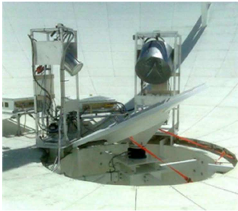
Fig. 1. Two feeds and tertiary mirror at the vertex of the main reflector.
