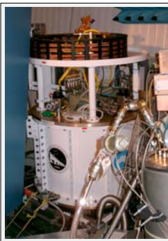
The 7-beam Arecibo L-Band Feed Array (ALFA) used in the Arecibo Ultra Deep Survey (AUDS). The array is situated at the Gregorian focus of the telescope and was installed in May 2004. The frequency range extends down to 1225 MHz, allowing HI observations to a redshift of 0.16.
