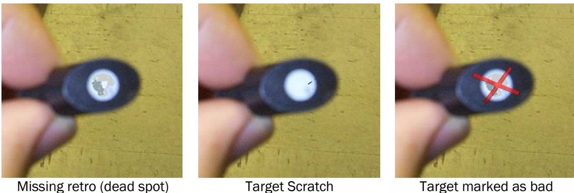
Figure 51: Inspection and treatment of obviously bad targets.
