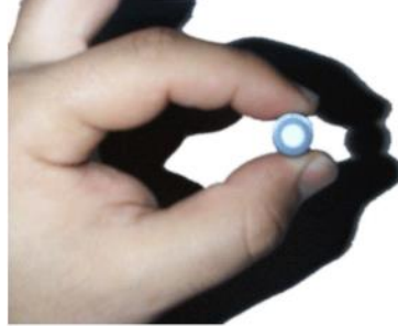
Figure 52: Correct retro target handling.
