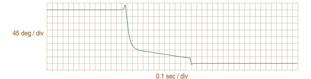
Phase history of typical disturbance of reference lock of chained PDEV synthesizers, measured at output of 3rd unit in the daisy chain. This example shows a single cycle slip; many disturbances manage to recover without any cycle slip.
