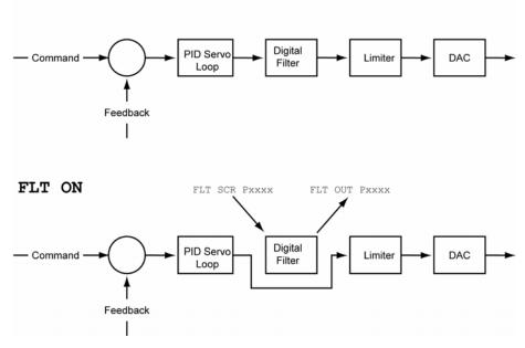
**NOTE:** This filter is still updated in the servo loop block. The sequence in which the input, output and digital filter will update should be carefully sought, so that nothing is overwritten.
