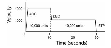
ACC 1000 DEC 1000 STP 0 VEL 1000 X/10000 : REM move 10,000 incremental units STP1000 VEL500 X/10000 : REM move 10,000 incremental units
