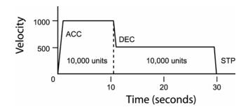
DEC 1000 ACC 1000 STP0 VEL1000 X/10000 : REM move 10,000 incremental units STP1000 VEL500 X/10000 : REM move 10,000 incremental units
