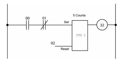
The following PLC code fragment implements the ladder logic as shown in the illustration above. Lines 100 and 110 create the first block. Line 130 connects the two blocks to counter 1, set the reset input to 2, and sets the count to 5. Line150 connects the counter output to relay 32.
