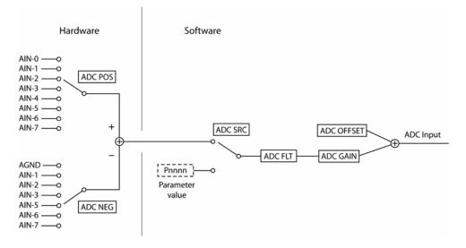
*Parameter value* in the above drawing is any system parameter (P4096 and up). The switch at ADC SRC is in the NONE position (using onboard ADCs).
