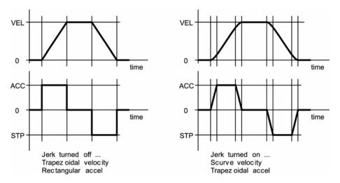
The following illustrates the result of using s-curve jerk on a normal move:
