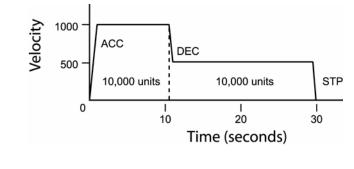
DEC 1000 ACC 1000 STP0 VEL1000 X/10000 : REM move 10,000 incremental units STP1000 VEL500 X/10000 : REM move 10,000 incremental units
