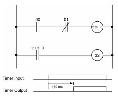
The following PLC code fragment implements the ladder logic shown above. Lines 100 and 110 create a new logic block. Line 120 connects the block to timer 0 and sets the timer to 150 milliseconds. Lines 130 and 140 connect the timer output to relay 32.
