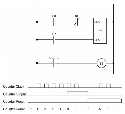
The following PLC code fragment implements the ladder logic as shown in the illustration above. Lines 100 and 110 create the first block. Line 120 creates the second block. Line 130 connects the two blocks to counter 1 and sets the count to 5. Lines 140 and 150 connect the counter output to relay 32.
