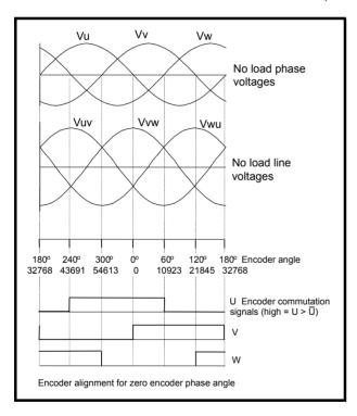
The encoder can be aligned statically by connecting the motor to a DC power supply as shown:
