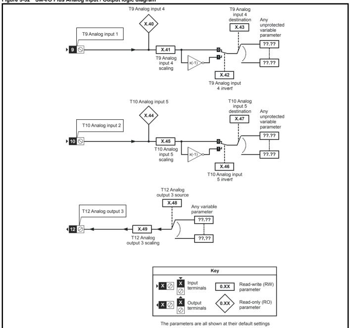
This module has two analog inputs (Al1 and Al2) and one analog output (AO1). The input operates in voltage mode only and the nominal full scale level is 9.8V. This ensures that when the input is driven from a voltage produced from the drive's own 10V supply, the input can reach full scale. The output operates in voltage mode only.
