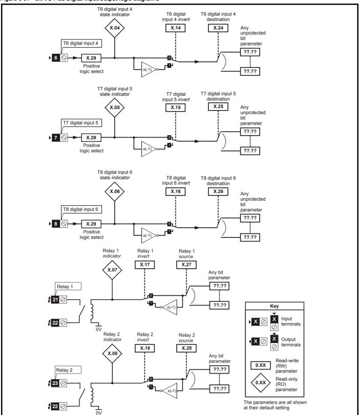
This module has three digital input/outputs (DI/O1 to DI/O3), three digital inputs (DI4 to DI6) and two relays outputs (D07 and DO8). The inputs can operate with positive or negative logic (defined by Pr x.29), the outputs operate with positive logic using high side drivers only and the relay outputs operate with positive logic only.
