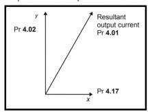
The resultant current magnitude is displayed by this parameter. The active current is the torque producing current for a motor drive and the real current for a regen unit. The reactive current is the magnetizing or flux producing current for a motor drive.
