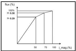
If Pr **5.29** and Pr **5.30** have their default values of 50 and 75, the characteristic becomes one line and there will be a linear relationship between the drive estimate of flux and the flux producing current. If Pr **5.29** and Pr **5.30** are increased above 50 and 75 the drive estimate of flux can include the effect of saturation. It is unlikely that information will be available to set up these parameters, and so the values are determined during the rotating auto-tune test.
