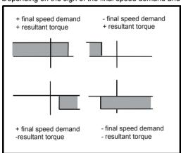
This mode of operation can be used where torque control is required, but the maximum speed must be limited by the drive.
