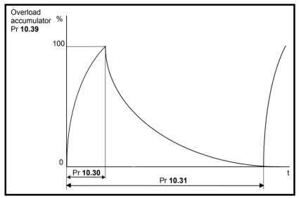
Assuming that the full power braking time is much shorter than the full power braking period i.e. Pr 10.30 < Pr 10.31 /10 (which is normally the case) the values for Pr 10.30 and Pr 10.31 can be calculated as follows:
