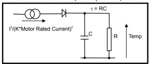
The temperature of the motor as a percentage of maximum temperature, with a constant current magnitude of I, constant value of K and constant value of motor rated current (set by Pr 5.07 or Pr 21.07) after time t is given by
