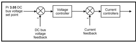
The gains of the voltage and current controllers affect the stability of the regen unit control system and incorrect gain settings can result in overvoltage or over-current trips. In many applications the default gains given for the current controllers (Pr **4.13** and Pr **4.14**) will be suitable, however, it may be necessary for the user to change these if the inductance or resistance of the supply plus the regen inductors varies significantly from the expected values.
