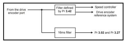
The diagram above shows the filter arrangement. It should be noted that the same filtering is provided at the speed controller input and for Pr 3.02 when the feedback is obtained from a Solutions Module, but the variable length window filter is controlled by Pr x.19.
