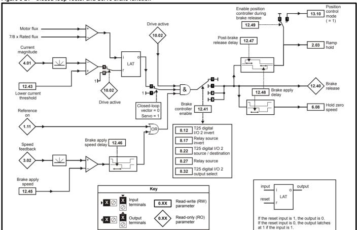
Figure 5-22 Closed-loop vector and Servo brake sequence
